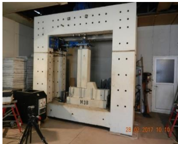
Fig. 10. Set-up of 1/2 scaled model M3-B in referent testing frame
