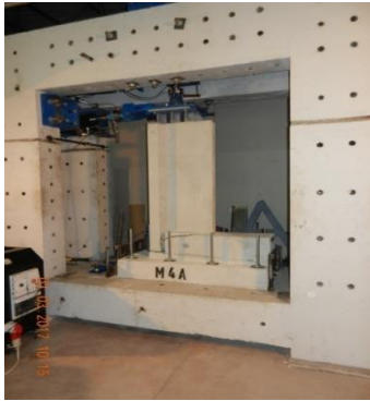
Fig. 13. Set-up of 1/2 scaled prototype model M4-A
