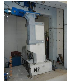
Fig. 6. Loading of RC corbel using rubber pad
