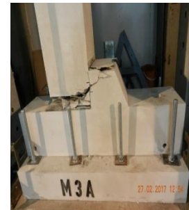
Fig. 9. Final failure state of original connection M3-A
