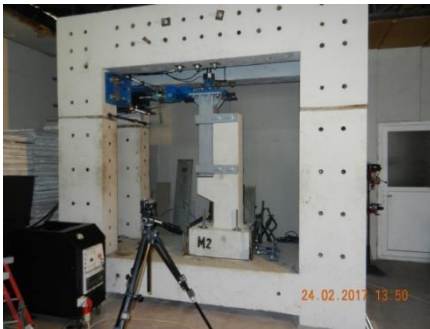
Fig. 4. Set-up of 1/2 scaled prototype model M2 in laboratory testing frame
