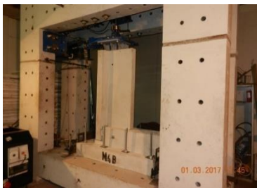
Fig. 16. Set-up of 1/2 scaled model M4-B in testing frame
